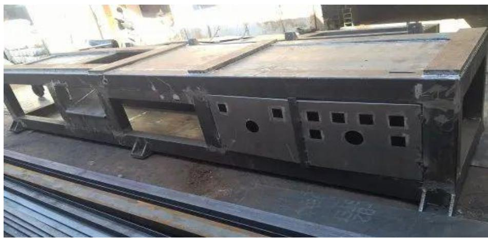
19. Once these sub-assemblies are manufactured, injection unit and clamping units are assembled to make complete machine. These sub-assemblies are mounted onto the machine frame and integrated with hydraulic and electrical systems. Control system is then installed to manage the machine's operations.
