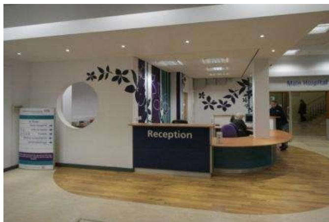
Photo 6-1. Reception with adequate illumination, two levels and colour contrast
